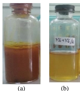
Figure 2: Off Grade CPO from: (a) Before Refinement and After Refinement.
