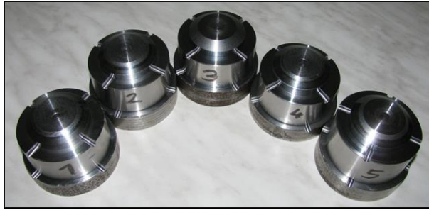
Figure 10: Molds prepared for 5 different cone heights
