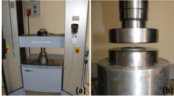
Figure 3: a) Compression test device on which the tests were applied b) Appearance of the disc spring on the compression test device
