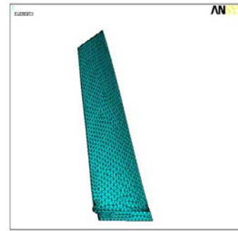
Fig.1. FEM model of a DD6 blade
