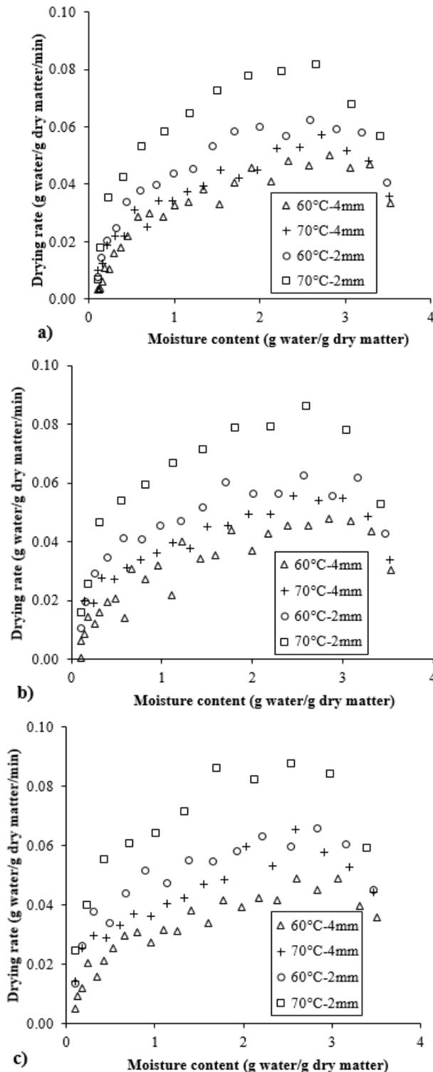
Figure 2: Drying rate changes of potato slices with pre-treatment by (a) Control; (b) US 20; and (c) US 40.
