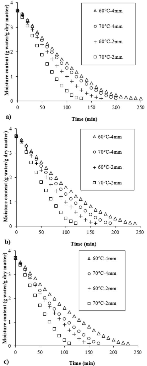
Figure 1: Drying curves for convective dried potato slices with pre-treatment by (a) Control; (b) US 20; and (c) US 40.
