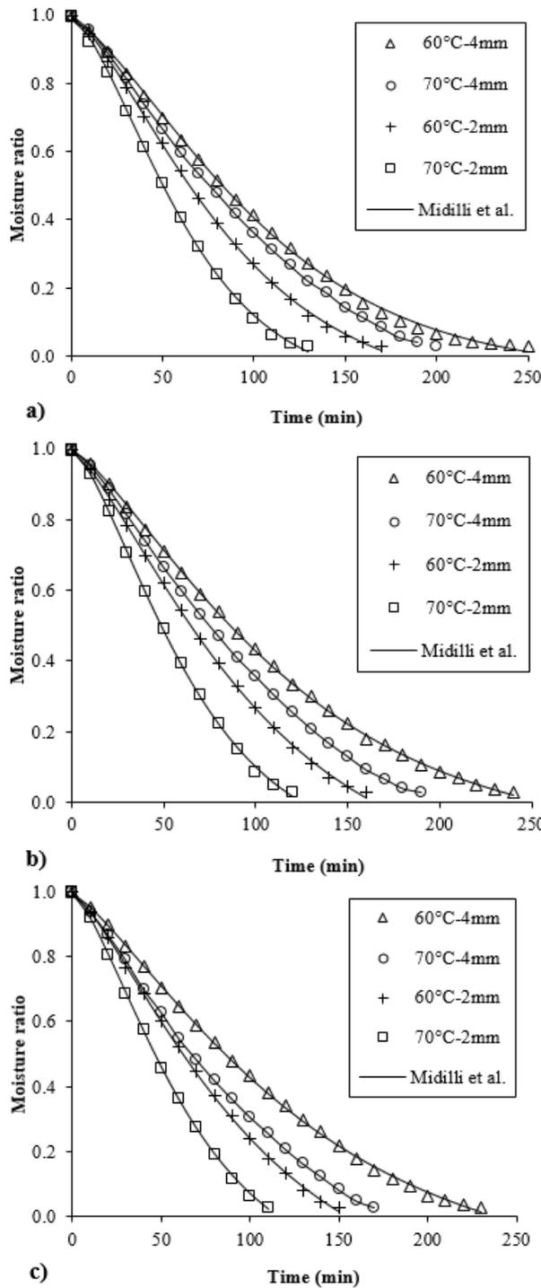
Figure 3: Comparison of the best model to experimental moisture ratios of potato slices with pre-treatment by (a) Control; (b) US 20; and (c) US 40.
