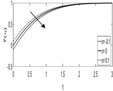
Fig. 6: Velocity distribution against  $\eta$  for various values of  $c$  when  $K = 0.1, M = 0.1, A = 0.1, Pr = 1.0, E = 0.1$  ( $n < 1$ ).
