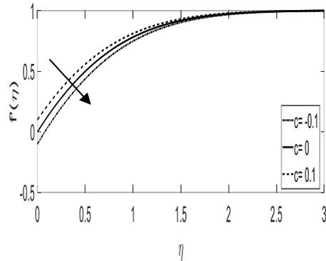
Fig. 7: Velocity distribution against  $\eta$  for various values of  $c$  when  $K = 0.1, M = 0.1, A = 0.1, Pr = 1.0, E = 0.1$  ( $n > 1$ ).
