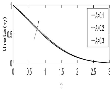
Fig. 10: Temperature distribution against  $\eta$  for various values of  $A$  when  $K = 0.1, M = 0.1, Pr = 1.0, c = 0.1, E = 0.1$ .
