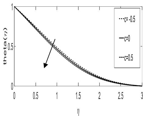
Fig. 9: Temperature distribution against  $\eta$  for various values of  $c$  when  $K = 0.1, M = 0.1, A = 0.1, Pr = 1.0, E = 0.1$  ( $n > 1$ ).
