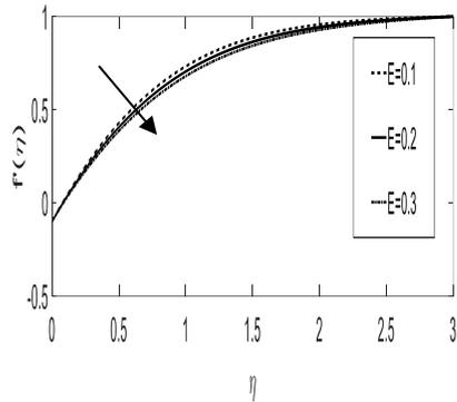
Fig. 4: Velocity distribution against  $\eta$  for various values of  $E$  when  $K = 0.1, M = 0.1, A = 0.1, Pr = 1.0, c = -0.1$  ( $n < 1$ ).
