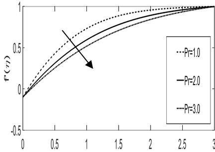
Fig. 3: Velocity distribution against  $\eta$  for various values of  $Pr$  when  $K = 0.1, M = 0.1, A = 0.1, E = 0.1, c = -0.1$  ( $n > 1$ ).
