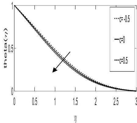
Fig. 8: Temperature distribution against  $\eta$  for various values of  $c$  when  $K = 0.1, M = 0.1, A = 0.1, Pr = 1.0, E = 0.1$  ( $n < 1$ ).
