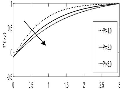
Fig. 2: Velocity distribution against  $\eta$  for various values of  $Pr$  when  $K = 0.1, M = 0.1, A = 0.1, E = 0.1, c = -0.1$  ( $n < 1$ ).
