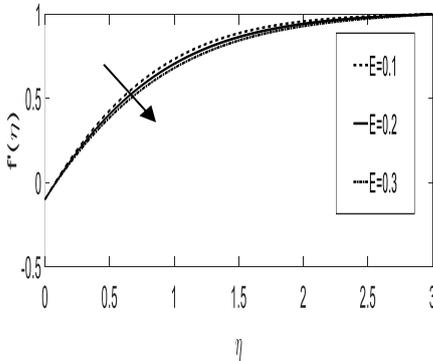
Fig. 5: Velocity distribution against  $\eta$  for various values of  $E$  when  $K = 0.1, M = 0.1, A = 0.1, Pr = 1.0, c = -0.1$  ( $n > 1$ ).
