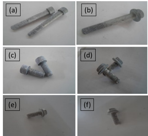
Figure 6: Bolt samples after salt spray test (a) M8*2-layers (720 hours) (b) M8*3-layers (1008 hours) (c) M10* 2-layers (720 hours) (d) M10* 3-layers (1008 hours) (e) M12* 2-layers (720 hours) (f) M12* 3-layers (1008 hours).
