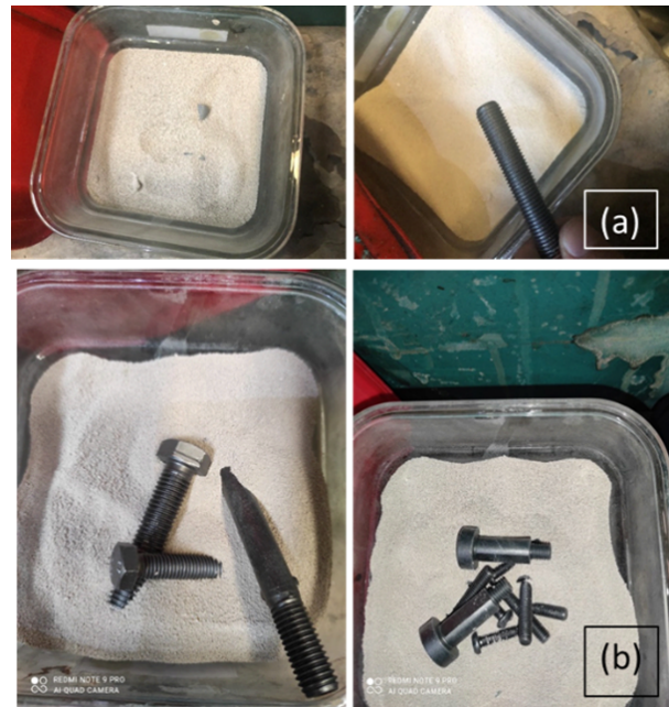
Figure 2: Zirblast test results (a) sandblasted with S70 sand (b) sand-blasted with S20 sand.
