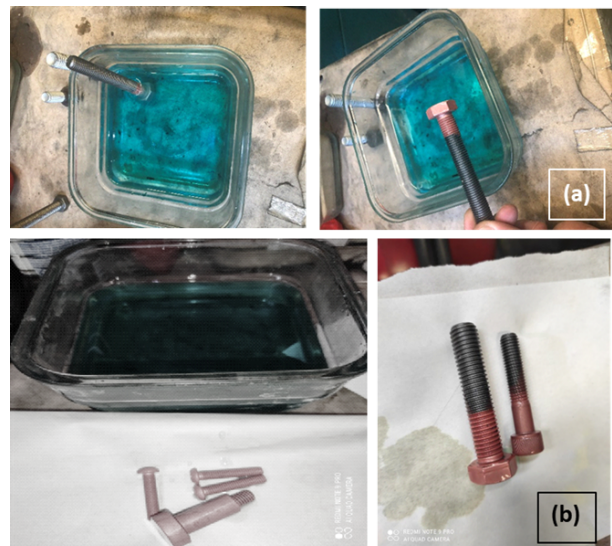
Figure 3: Hogaboom test results (a) sandblasted with S70 sand (b) sandblasted with S20 sand.
