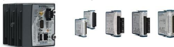
Figure 3. CompactRIO controller and its I/O boards
