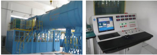
Fig. 8. Wind tunnel of aerodynamic experiments for the conductor
